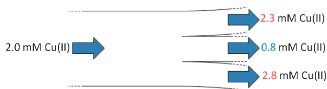
Figure 3. Extraction of Cu(II) from the homogeneous ternary mixed solution into the outer phases in the side narrow channels through TRDP. Conditions: Carrier, water–acetonitrile–ethyl acetate (2:3:1, v/v/v) mixture; flow rate, 40 \mu\text{L min}^{-1} for channel W; initial Cu(II) concentration, 2.0 mM.
